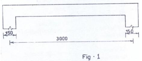
(i) Reproduce the sketch and show details of steel reinforcements in the slab and beams.
