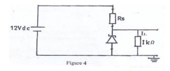
In Figure 4, a 5 V stabilised power supply is required from a 12 V d.c. input source. If the maximum power rating of the zener diode is 2 W, calculate the
