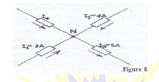
(b) (i) In Fig. 8, calculate the current I<sub>4</sub>;
